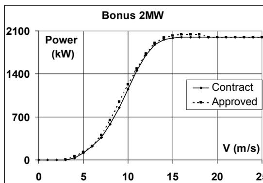
**Figure 6:** Power curve for the 2 MW turbines. Production figures can be found on [www.middelgrund.com](http://www.middelgrund.com). The information is updated every 10 minutes
